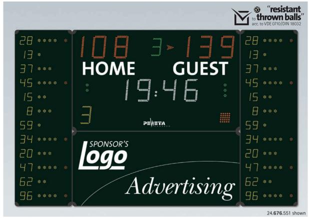
Game result displays/scoreboards, in 7-Segment LED display technology, composed of a main scoreboard and two 12-line foul displays. As a stand-alone-unit, the main scoreboard is suited for most kinds of indoor sports. For basketball, the two augmenting displays show player numbers and the number of their personal fouls.
