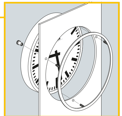
Installation inside a media pillar by means of a front ring (extra)
